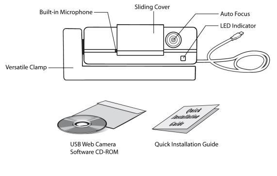
• Note: 1. The power supply for the camera is provided through the USB cable.
